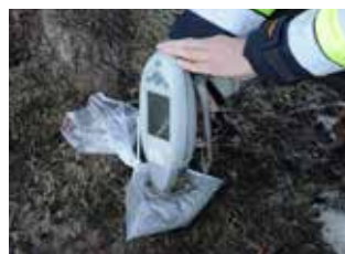
July 2013. As well as monitoring the water quality, regular soil samples are taken to be analysed both on the spot and in a laboratory.
